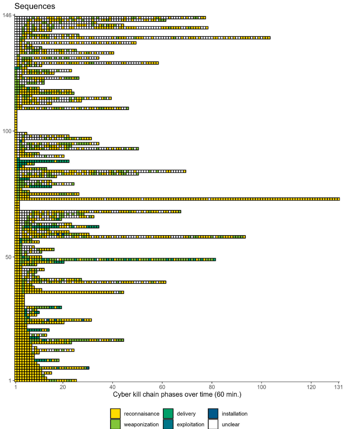
Fig. 2. Participants' hacking sequences according to the phases of the cyber kill chain.
